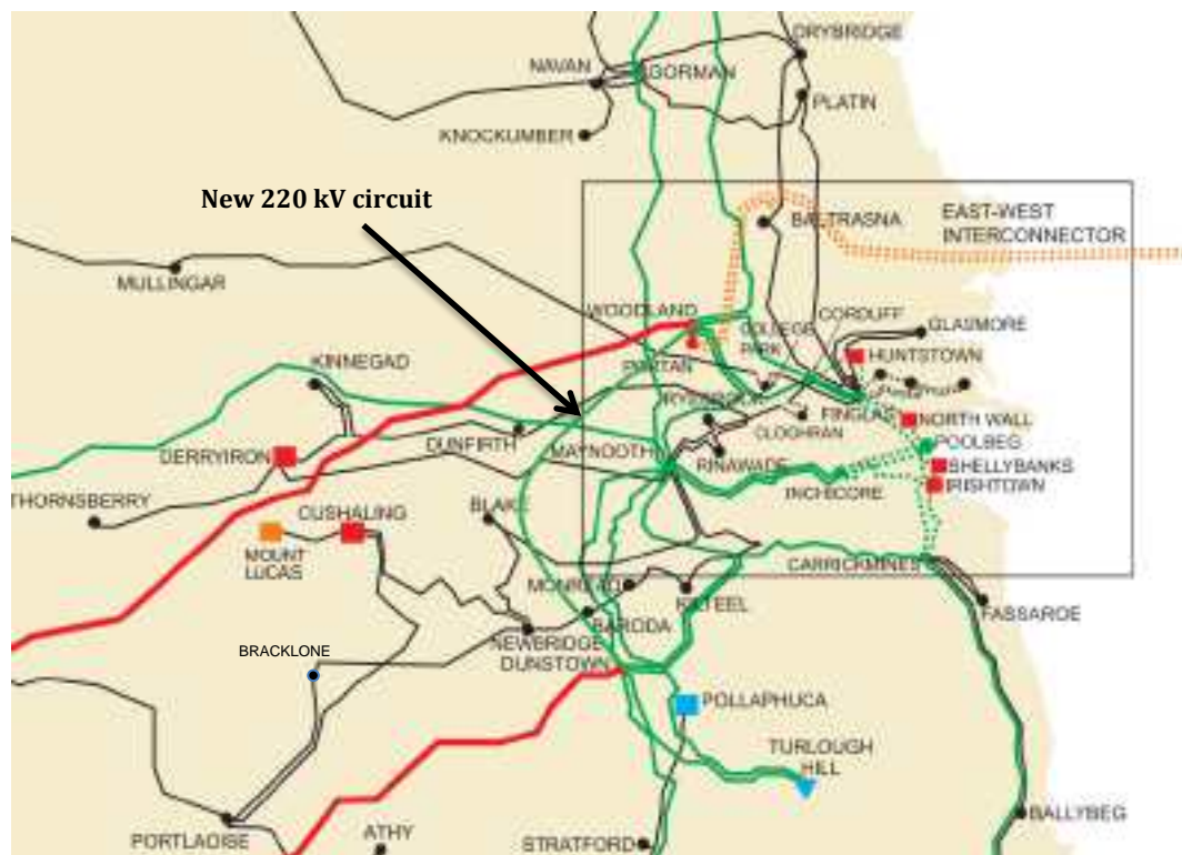
Figure 5 Transmission system map showing a new 220 kV OHL (indicative) (the 220kV OHL between Dunstown and Woodland 400kV stations are shown as a green bow, in a north southerly direction)
