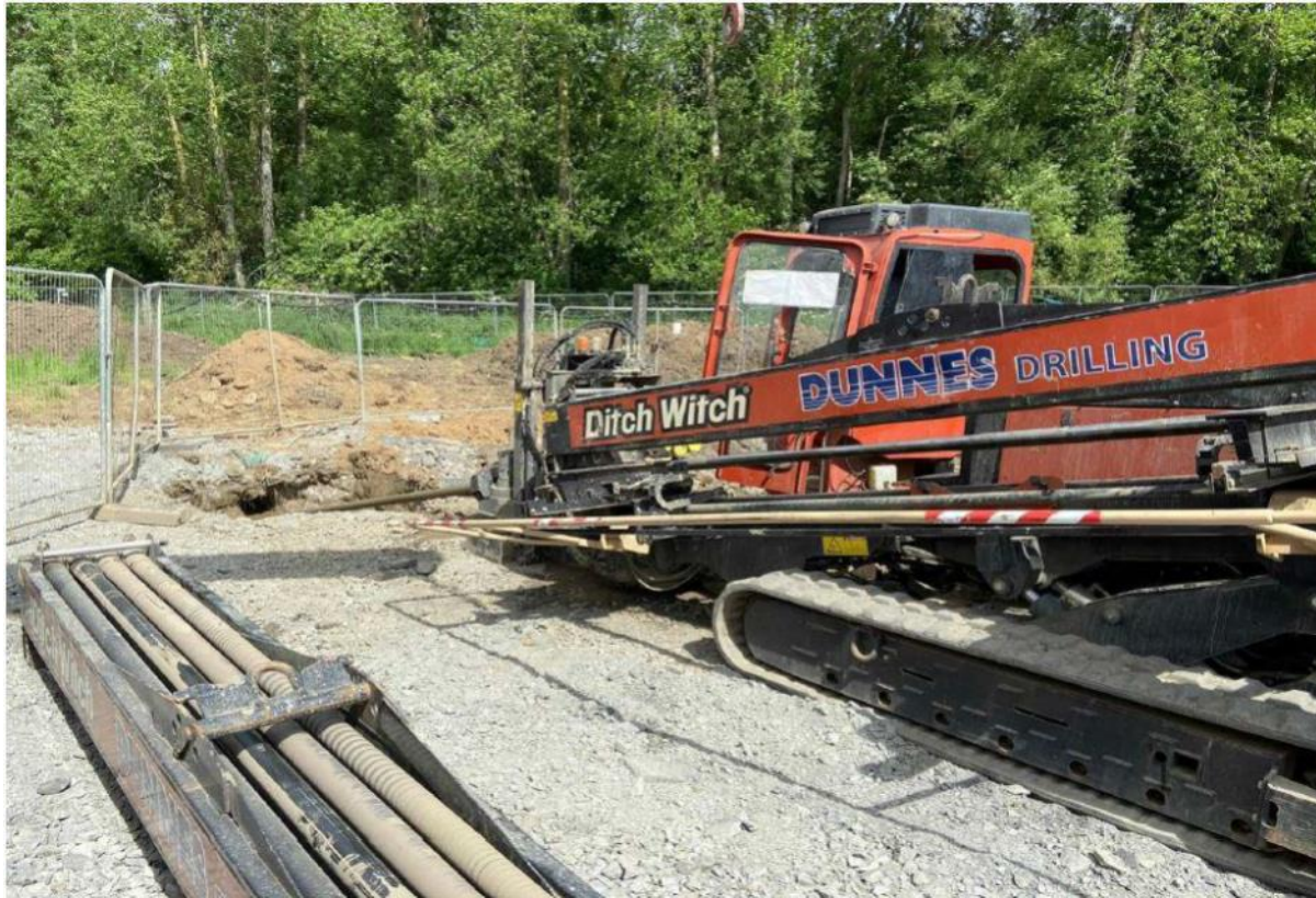
Plate 5.13: Typical HDD Drilling Rig
